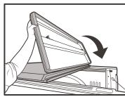
Holding mid and tail panels tightly together, begin unfolding towards tailgate.
