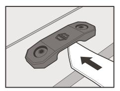
Feed straps underneath anchor plates.
