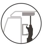
Thoroughly compress the weatherstrip by applying a significant amount of downward pressure to the tail panel and engage the clamp. The clamp tension should be firm enough to clamp the cover
