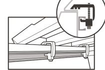
Release the handle from the track and position clamp jaw inside track to begin engaging.
