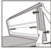
Lift tail panel and fold to mid panel. While holding tightly together, fold on to cab panel.
