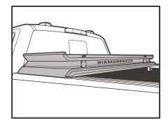
Apply force towards the tailgate at the double-hinge area when folding and unfolding the mid panel. Do not lift directly upwards at the hinge area. Let gravity assist in folding/unfolding.
