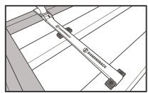
Carefully unfold the cover towards the tailgate by applying force at the double-hinge area and allowing gravity to assist with unfolding.
