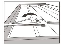
Pull strap tight and make sure buckle is securely engaged
