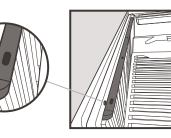
Clean the bottom of the bulkhead bar thoroughly with a clean, lint-free cloth and rubbing alcohol. Allow to dry.
