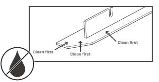
Affix the **gasket** to the bottom of the bulkhead bar:
