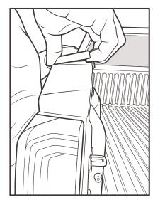
Using upward force, continue working towards the cab releasing clips until you have completely removed one of the bed rail caps from the truck.
