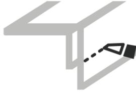
**10** If your bed rail lips have sharp edges, they might tear the rubber caps on the ends of the tailgate-panel lock rods. To protect the end caps, peel the red adhesive backing from the **bed-rail edge trim** pieces, then affix one piece to each on the bed rail lips where the tailgate-panel lock rods pass underneath.
