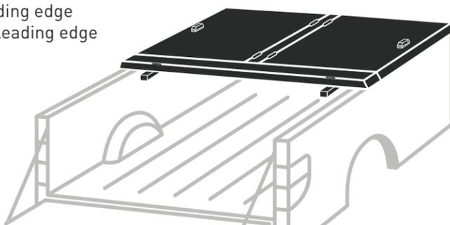
**5** Slide the tailgate panel onto the T panel by mating their hinges. Close the tailgate panel slowly while holding the lock handle in the open position.
