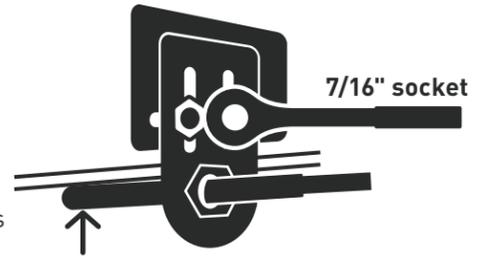
**!** To get the weatherstrip compression necessary for its adhesive to cure and the cover to keep out the weather, have a second person press down on the cover while you're adjusting the lock rods.
