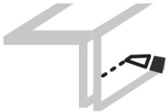
**9** Peel the red adhesive backing from the bed-rail edge trim pieces. Affix one piece of trim to each of the newly cut-out, exposed metal areas of the bed rail.
