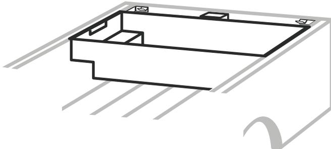
Many pickup truck cargo beds are tapered, which means that many Cross Bins have a front and back. If your bin appears to not fit, rotate it 180° and try again.
