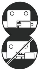
**7** If you just installed a the bin under a DiamondBack cover you've had for a while, you may find that your cab-panel lock rods are now more difficult to operate. If so, use the rod guide brackets and a 7/16" socket to lower the rods slightly.
