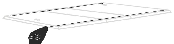
**6** Take a **long adapter bar** and insert one of its bolts through a stainless washer, through a foam washer, then into an open hole.
