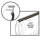
Thoroughly compress the weatherstrip by applying a significant amount of downward pressure to the tail panel and engage the clamp. The clamp tension should be firm enough to clamp the cover
