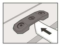
Feed straps underneath anchor plates.
