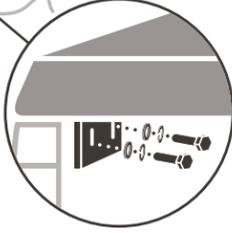
**!** To ensure a tight seal, it is crucial to apply downward pressure on the cover while you're attaching the mounting brackets.
