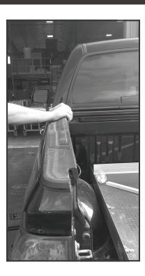
Standing at the tail and working cab-ward, use one hand as a wedge to pop out each remaining retainer clip one by one.
