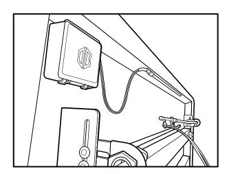
The mounting location must provide access to the battery compartment. There must be room to open the tabs and swing the battery door around 90°.
